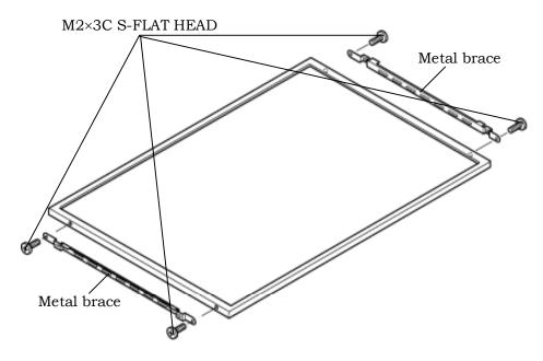
Figure 4-41 Removing the LCD module (2)
